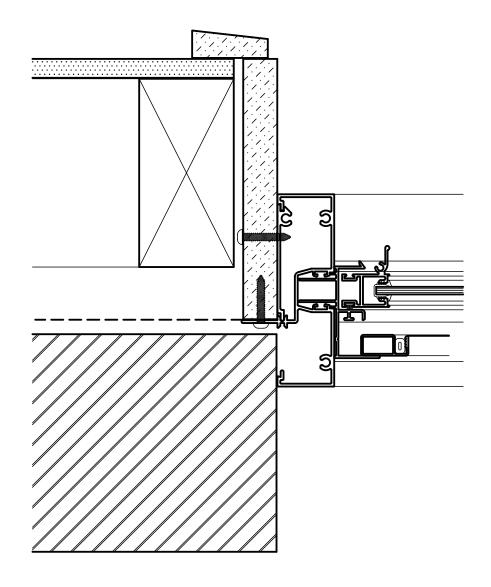
Standard 30mm Nailing fin jamb into brick veneer wall.
