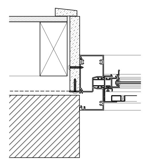
Alternative 44mm Nailing fin jamb into brick veneer wall.
